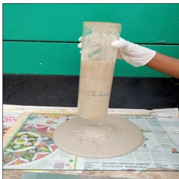
Flowability Measurement from the spread diameter
