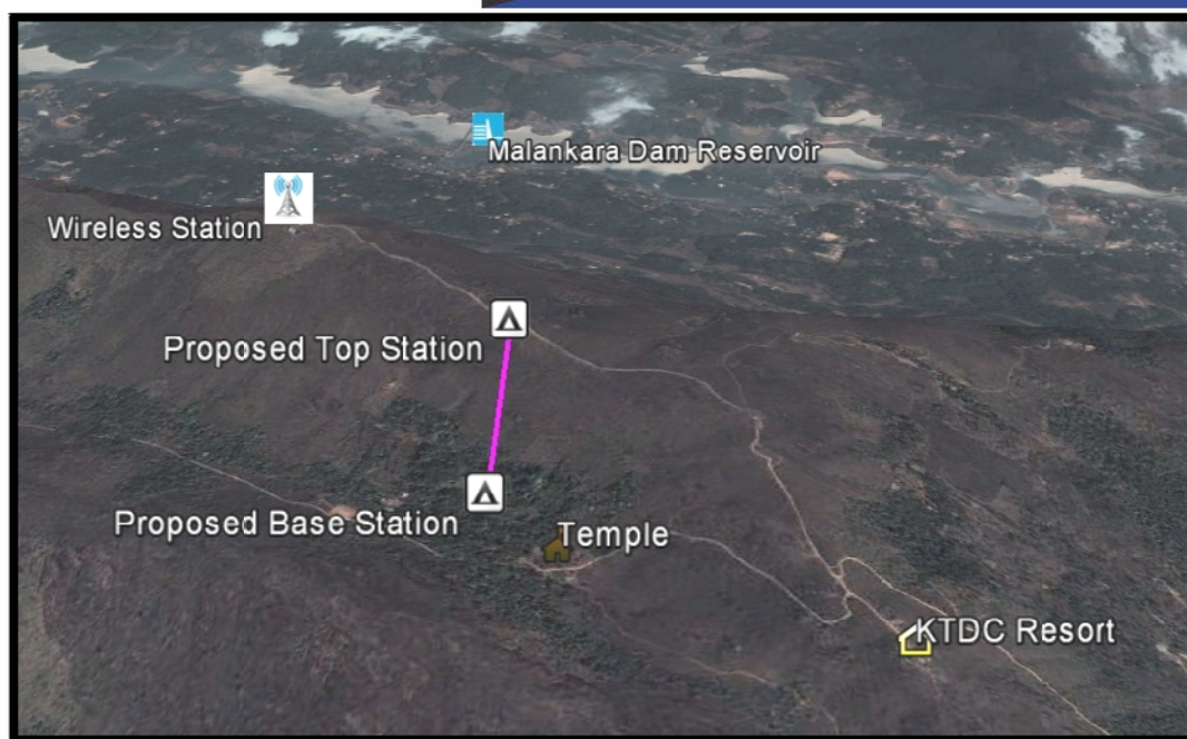
Figure 20: Proposed alignment for ropeway system
