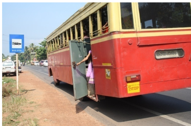
Plate 4 Bus Stopping at the Carriageway Due to Lack of Bus Bay
