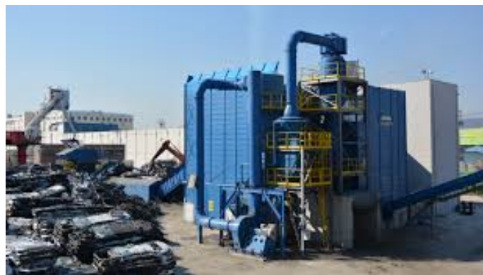
Plate 18: The main shredder (Capacity is 10 vehicles ie. car body size an hour)
