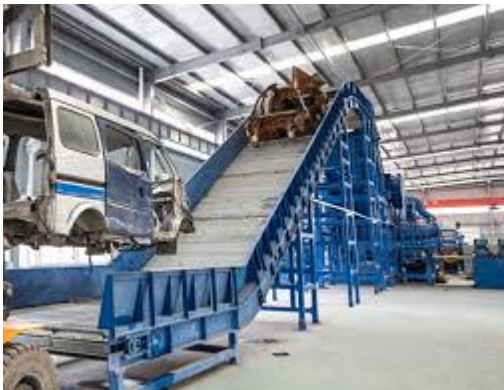
Plate 18: The main shredder (Capacity is 10 vehicles ie. car body size an hour)
